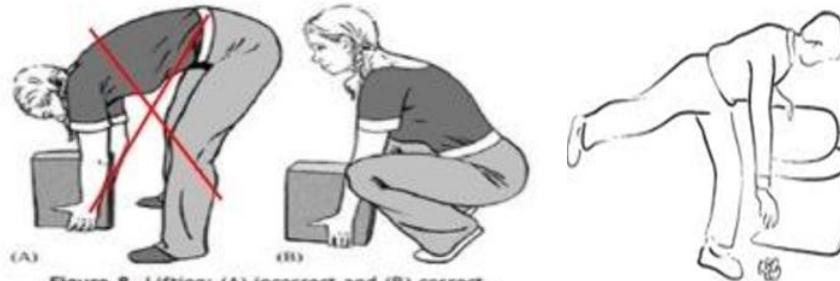
Figure 8 Lifting: (A) incorrect and (B) correct.
