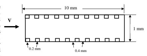
dispersion and deposition of particles in the range of 0.01 to  $10~\mu m$  from point sources located at three locations in the duct inlet. In addition, evaluate the deposition of particles for a uniform inlet concentration. (The flow is in the laminar regime.)
