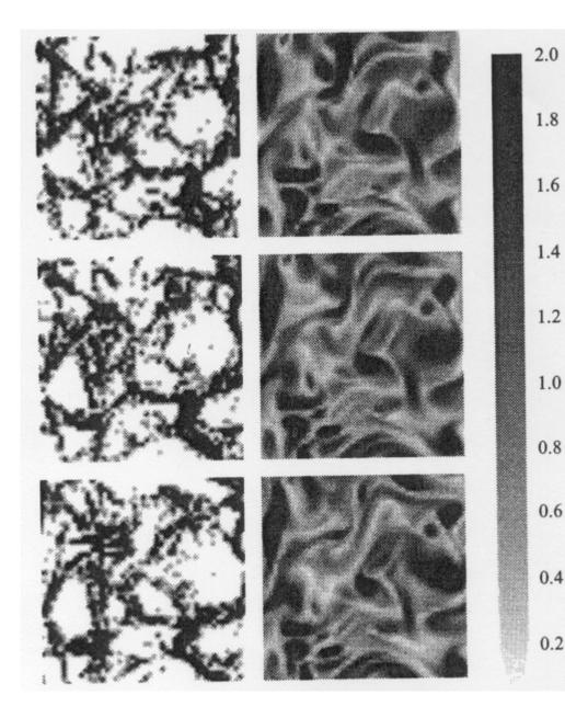
The particles may be seen on the left and the magnitude of the fluid vorticity is shown on the right. The particles are centrifuged out of regions of high vorticity into regions of low vorticity.
