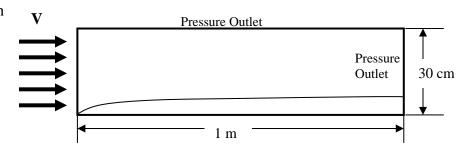
boundary layer thickness as a function of distance, and  $C_{\rm f}$  and  $C_{\rm D}$ .
