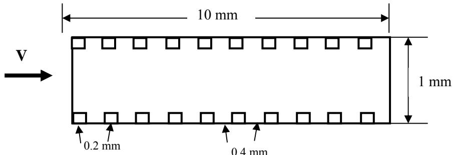
b) Assume that the elements are at temperature of 50°C and air at the inlet is at 20°C. Evaluate the temperature field for different flow rates. Also evaluate the net heat flux and the effective Nusselt number.
