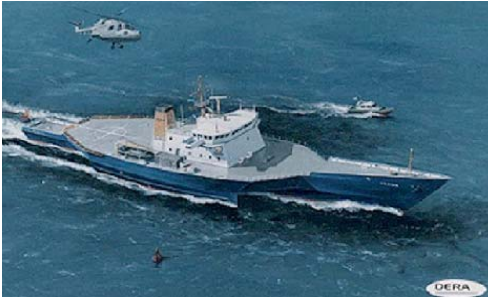
Figure 2: RV Triton, trimaran design test ship (GlobalSecurity.org, 2006)
