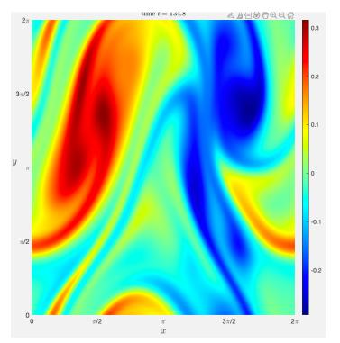
This data comes from an incompressible fluid, in a two dimensional square domain, as modeled by the Navier-Stokes equation stated in the same domain.
