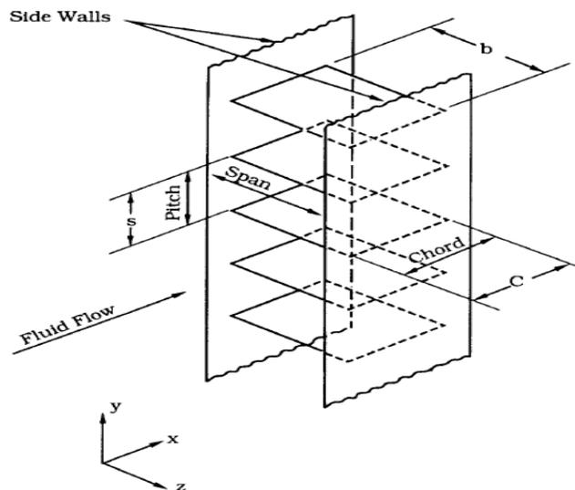
**Figure 14:** Flat Plate Cascade [4]
