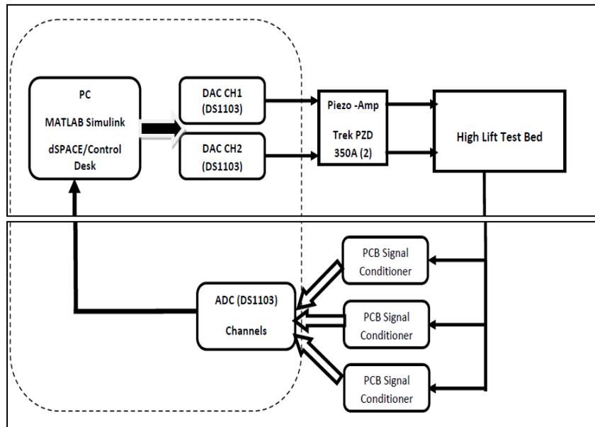
**Figure 5** Schematic of experimental setup
