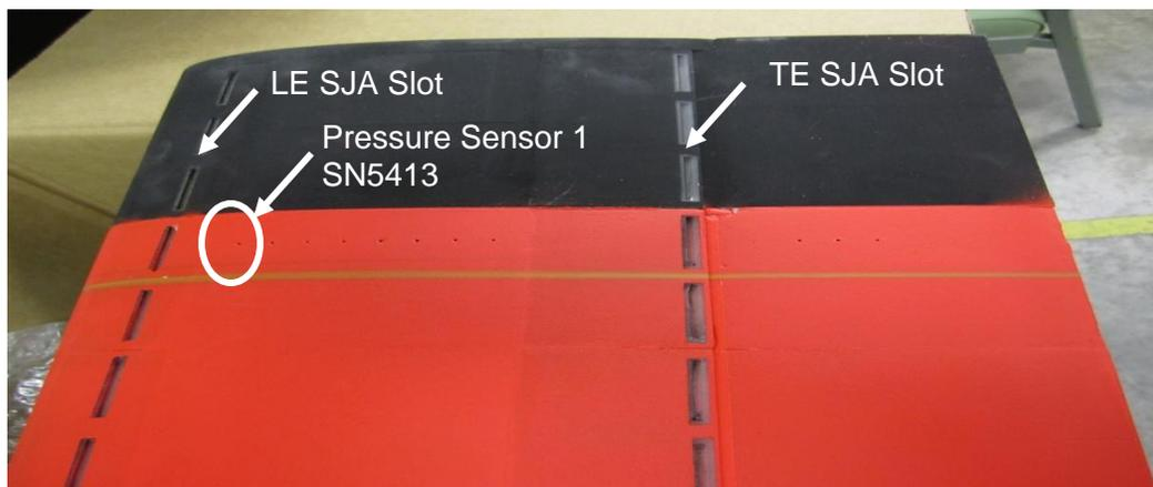
**Figure 7:** Location of Leading Pressure Transducer
