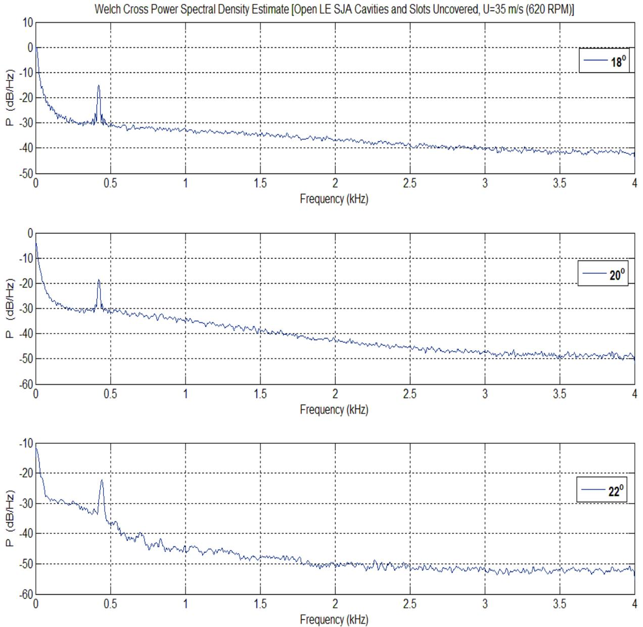
**Figure 11:** Pressure Spectra for AoA=18-22 degs
