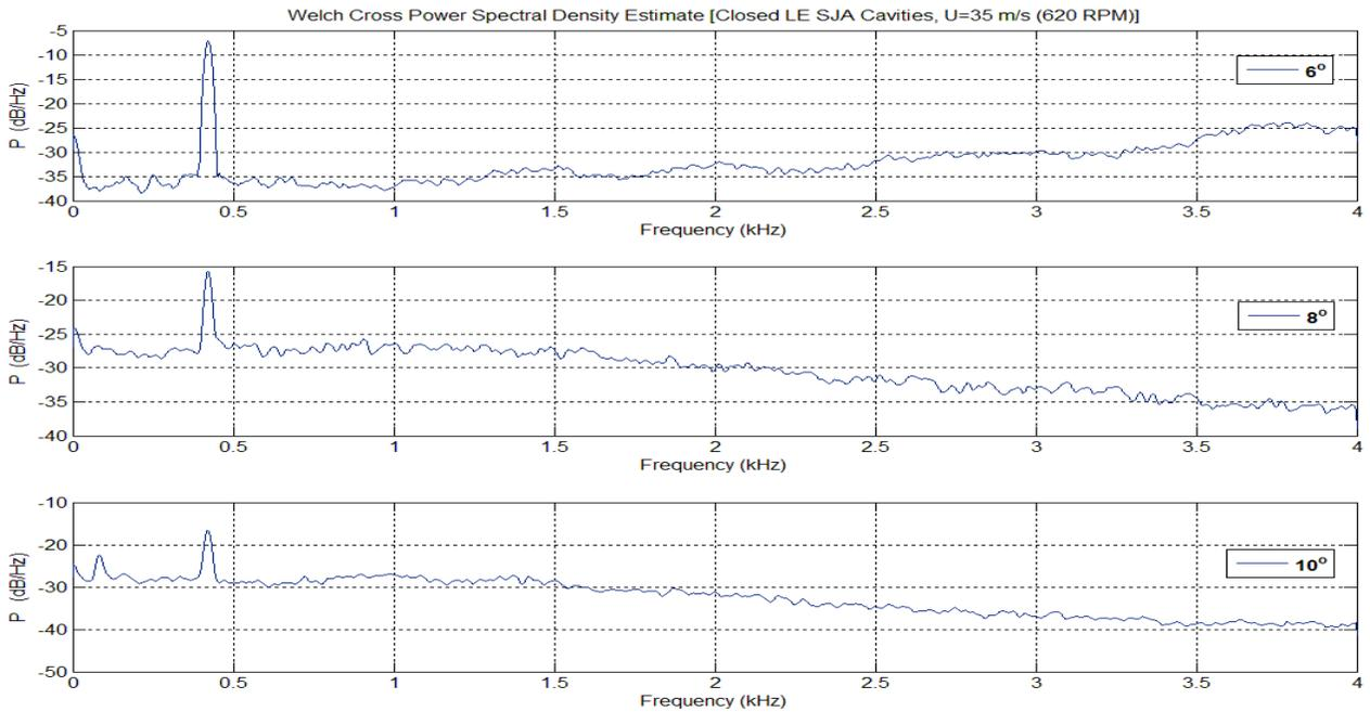
**Figure 13:** Pressure Spectra 6-10 deg AoA, Slots Covered
