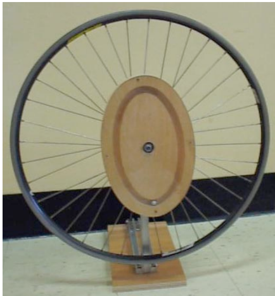
Fig. 7. Photograph of a physical model of ETT, built on a bicycle wheel, and a mounted piece of wood in which was routed the elliptical track. The white teflon ball shown moves freely and chaotically within the elliptical track. This wheel assembly is mounted on an inclining arm so that the effective strength of the gravity constant becomes g \sin \alpha , where \alpha is the angle at which the wheel is inclined from horizontal. \alpha = 90^\circ is shown in this picture.
