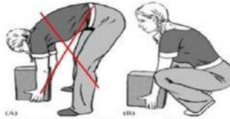
Figure 8 Lifting: (A) incorrect and (B) correct.
