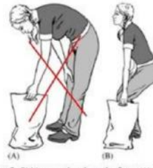
Figure 5 Picking up a bag from the floor: (A) incorrect and (B) correct.
