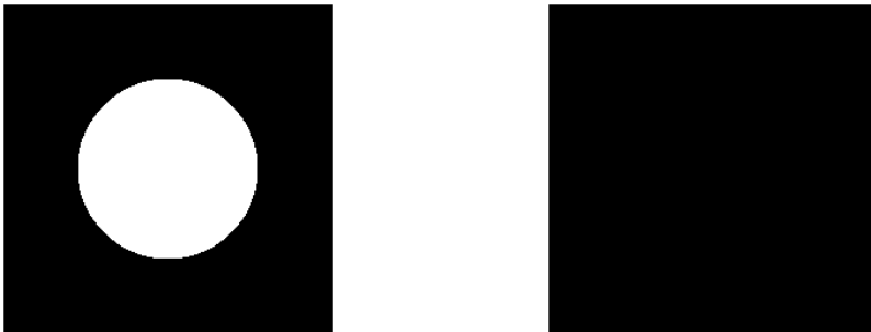
FIG. 8.2. The u part and v part of the image of circle in Figure 8.1 using uniform grid with h = 1 and \lambda = 0.0001 .
