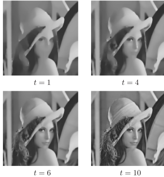
Figure 2. The images, U(t) = \int_0^t u(\cdot, s) ds , for the modified IDE (14) at t = 1, 4, 6, 10 . Here \lambda(t) = 0.002 \times 2^t .
